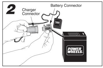
Squeeze the connector tabs on the charger connector and plug it into the battery connector.
